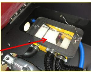
**Cover Off**: Reveals the metal grill to hold filter down and large white filter.
