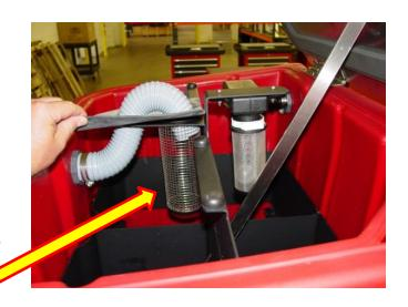
New Wider Bracket: This is part#: 370-1123 and it creates a barrier between the incoming dirty water hose from the squeegee and the stainless screen the float ball is inside. We found customers wouldn't properly install the hose into the drain saver basket.
