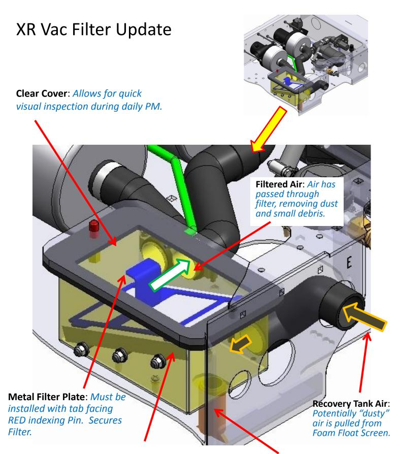
Disposable "white" Filter: Traps dust and foam pulled through Rec. Tank screen.
