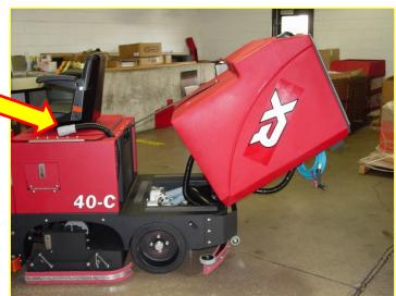
**New Hose Location:** The vacuum hose is missing from the front, and now installed at the rear of the tank. This makes tipping the tank back for service easier and reduces crushed hoses.
