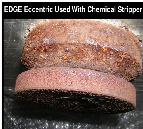
New Eccentric Test in Stripper for 90 hours
