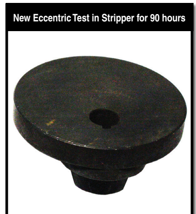
EDGE Eccentric Used With Chemical Stripper
